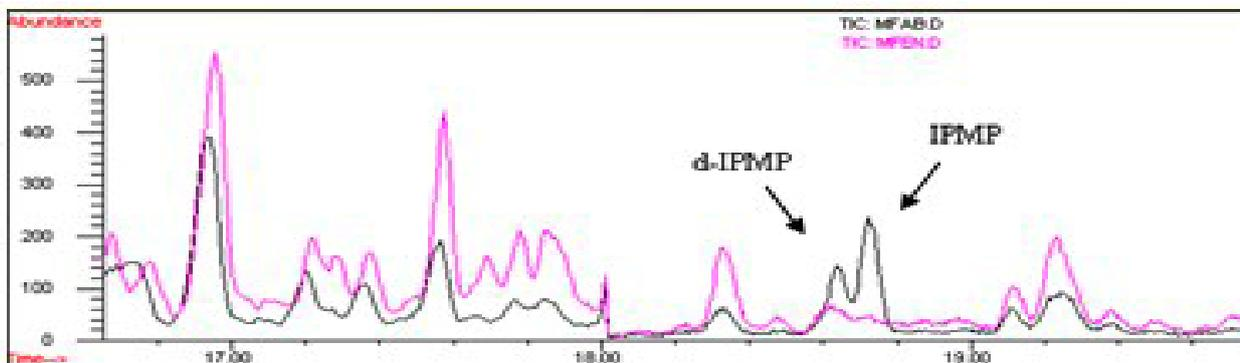
**Figure 3.1b** Indicative chromatogram for IPMP showing samples eluted with DM and EtAc. IPMP is identifiable only when it is eluted with DM. Both samples were concentrated under nitrogen stream to a final volume of 100 $\mu$ l.
