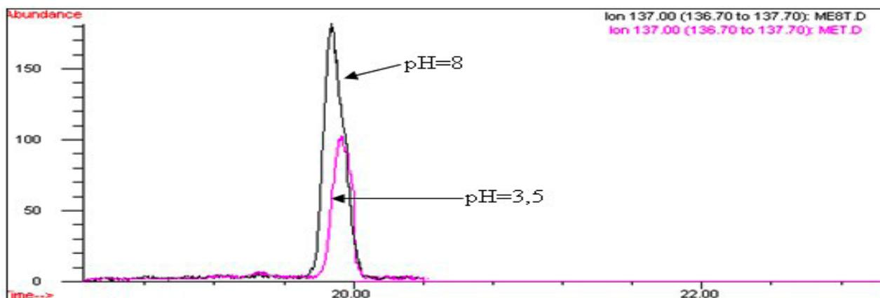
**Figure 3.1a** Indicative chromatogram for IPMP with sample pH adjustment from pH 3,5 to pH 8
