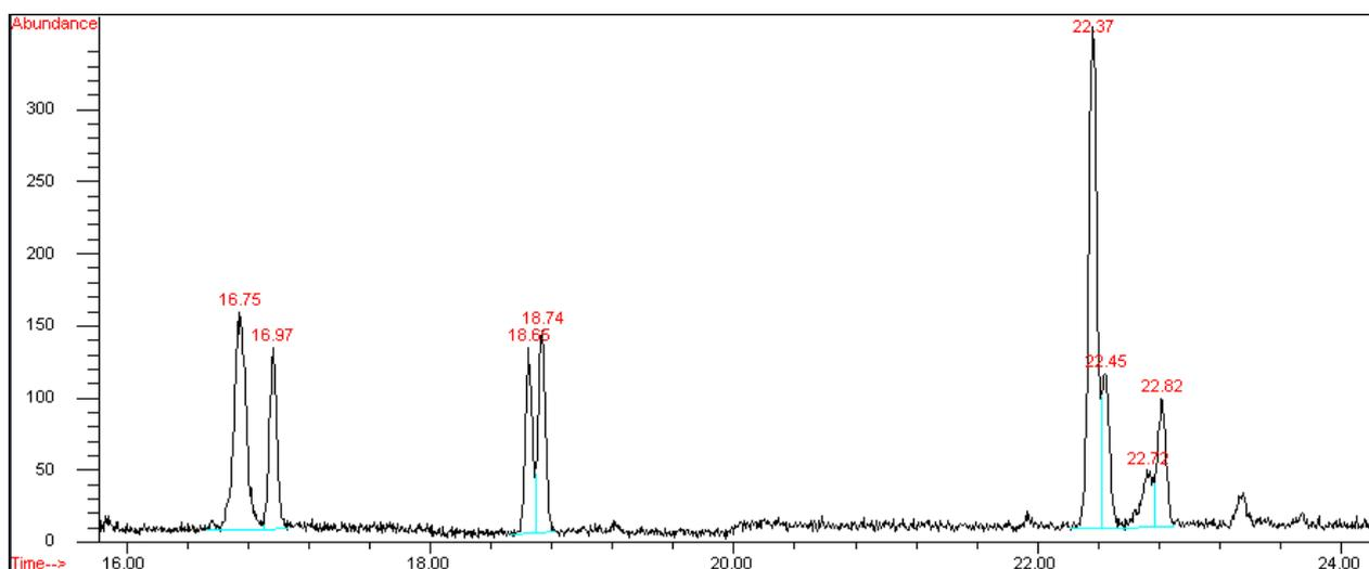
**Figure 2.3 Chromatogram of a standard solution containing all MPs in 10 $\mu$ g/L concentration. Each MP's retention time is marked on top of its respective peak.**
