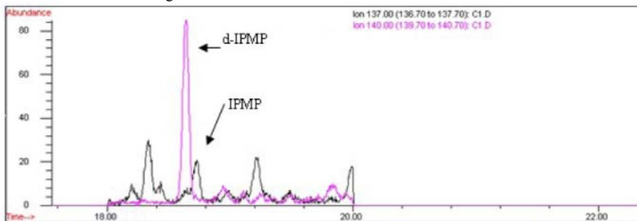
**Figure 2.5 Chromatogram of IPMP at 5 ng/L concentration after C-18 modified method including concentration of the sample under nitrogen stream.**
