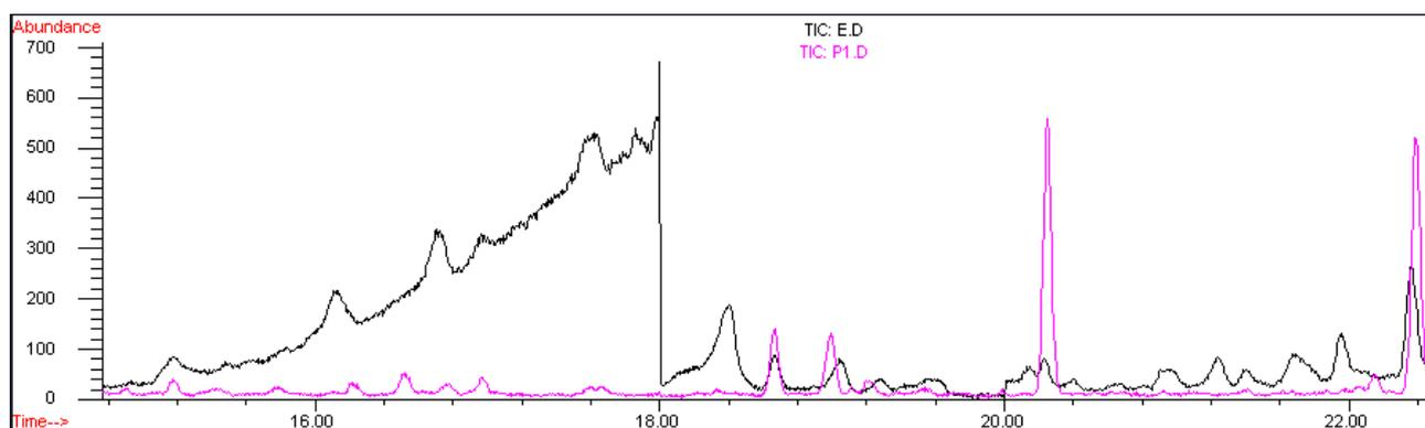
**Figure 3.1c** Overlapping chromatograms of samples were the clean-up solvent's volume were 25 and 50 ml. The clear peaks with less noise belong to the sample which was treated with the 50 ml.
